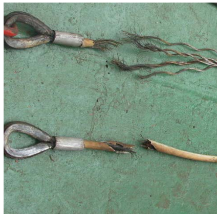
Figure 3. Lifting slings parted due to undetected corrosion.
