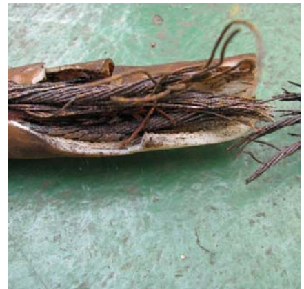
Figure 3. Lifting slings parted due to undetected corrosion.
