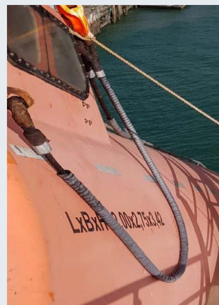
Figure 4. Alternative sheathing arrangement which allows for inspection
